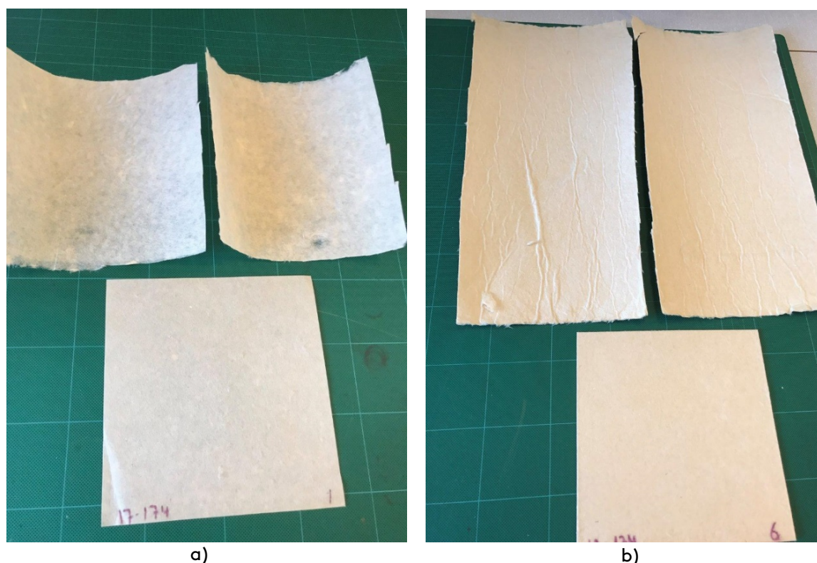
figure 9: lab sheets of a) Above: Sample 1 – First production cycle at STRATEX pilot-scale machine. Below: Sample 1 - Second production cycle as material at lab (lab sheet), and b) Above: Sample 6 – First production cycle at STRATEX pilot-scale machine., Below: Sample 6 - Second production cycle as material lab (lab sheet).
