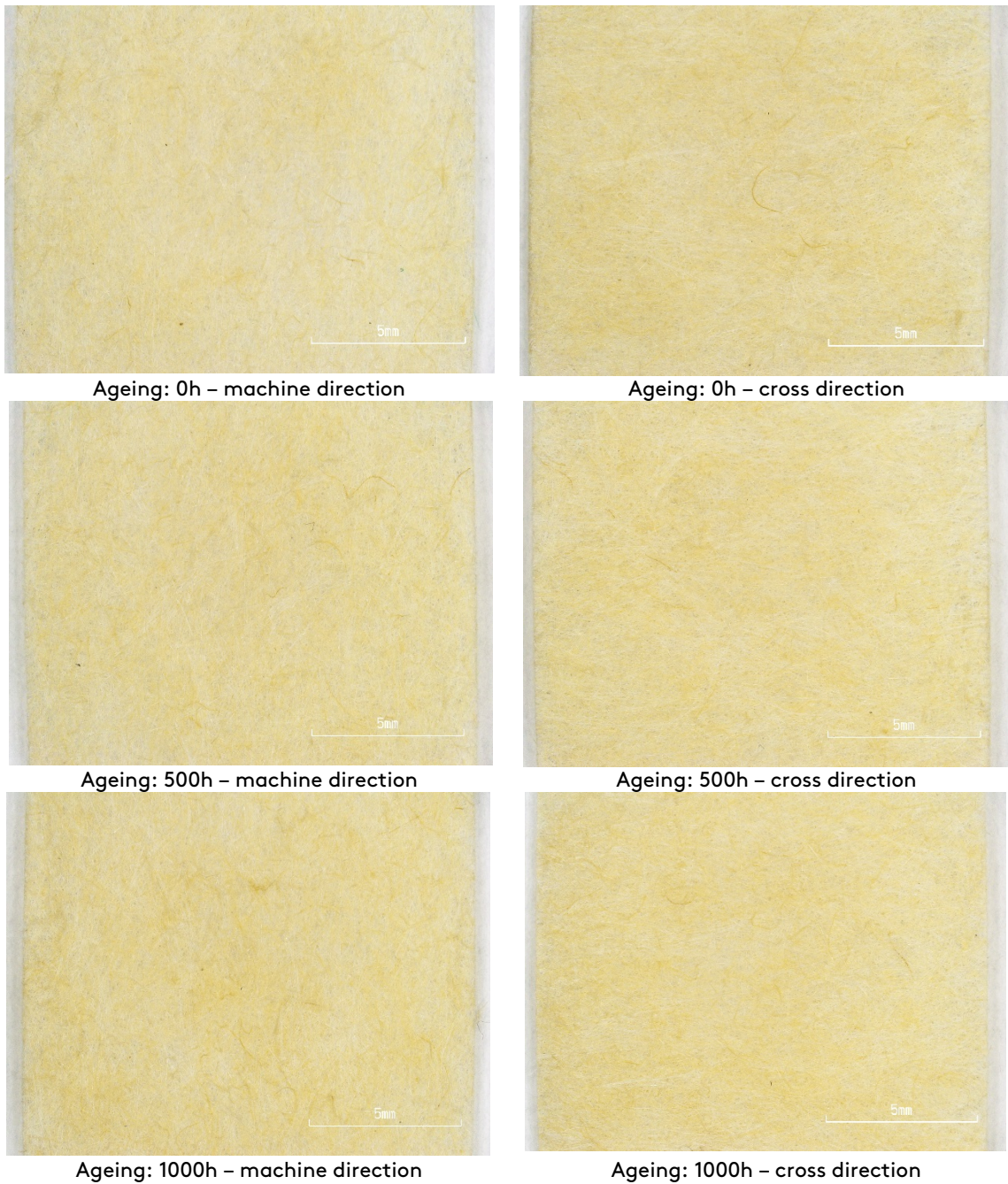
figure 10: Visual analysis of the aged material sample A-1 (grammage 42,4 g/m 2 ). Results from the screening accelerated ageing study.
