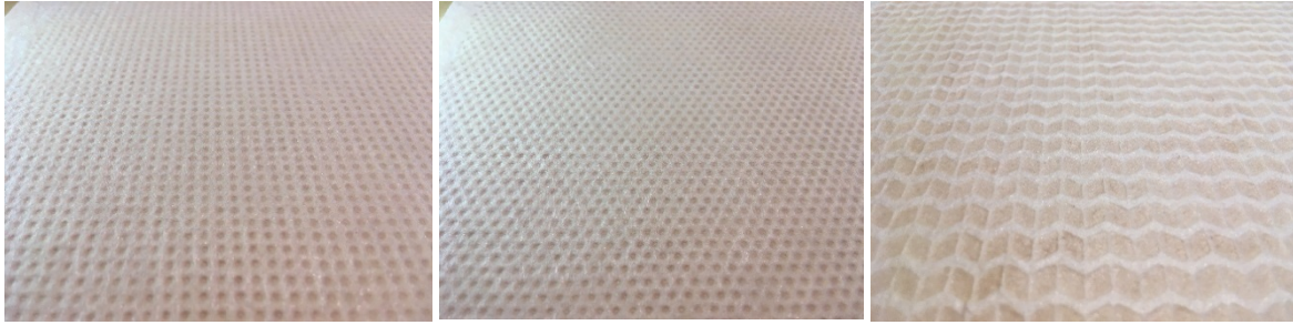
figure 2 The three different welding patterns that were used in the study. From left: square, zigzag, Miura welding patterns on A1 samples.
