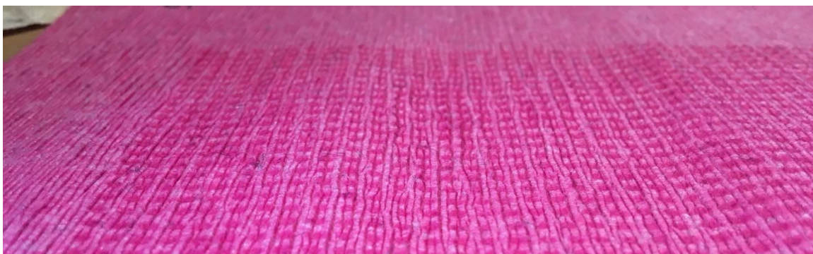
figure 4 Sample A2 showing left-right periodic undulations (~1mm) from industrial creping. The spot pattern comes from further welding treatment.
