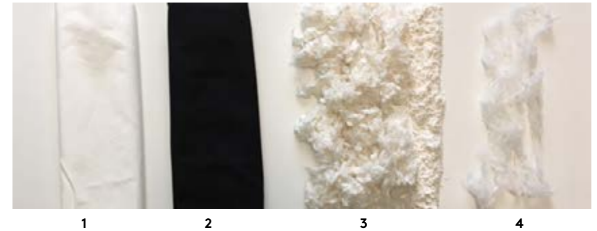
Figure 4: Materials after the process steps: 1) Original fabric 2) dyed fabric with or without textile finishes 3) decolourised pulp before and after grinding and 4) regenerated fibres.
