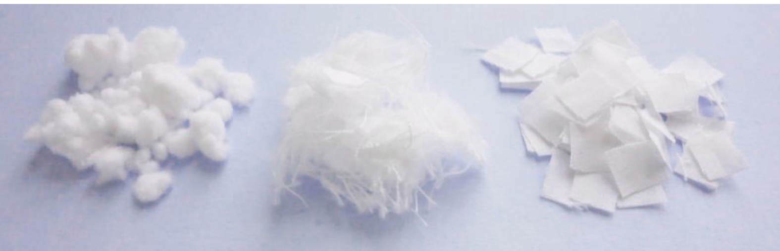
Figure 5 ground, shredded and cut material fineness of polycotton sheets. Picture by Stina Björquist.
