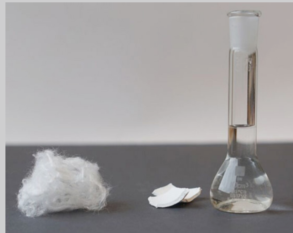
Three product streams from the process; viscose fibres, terephthalic acid and ethylene glycol.
