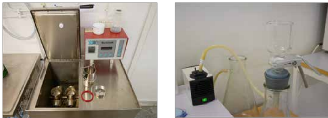
Figure 4. To the left the Gyrowash and to the right the filter equipment set-up for collecting the fibres in the waste water.
